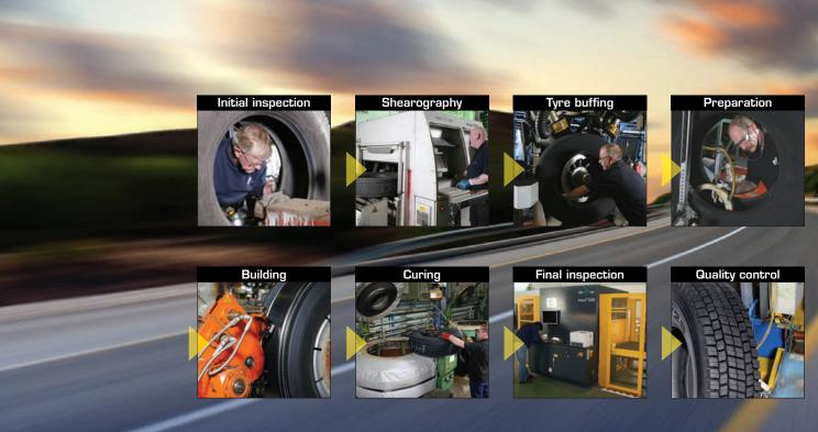
The Lodge Retreading Process involves taking a worn casing of good structure and quality and completely renewing the tread and the sidewall rubber. The rebuilt tyre then goes through a curing process during which the new rubber is vulcanised and the tread pattern is formed.
